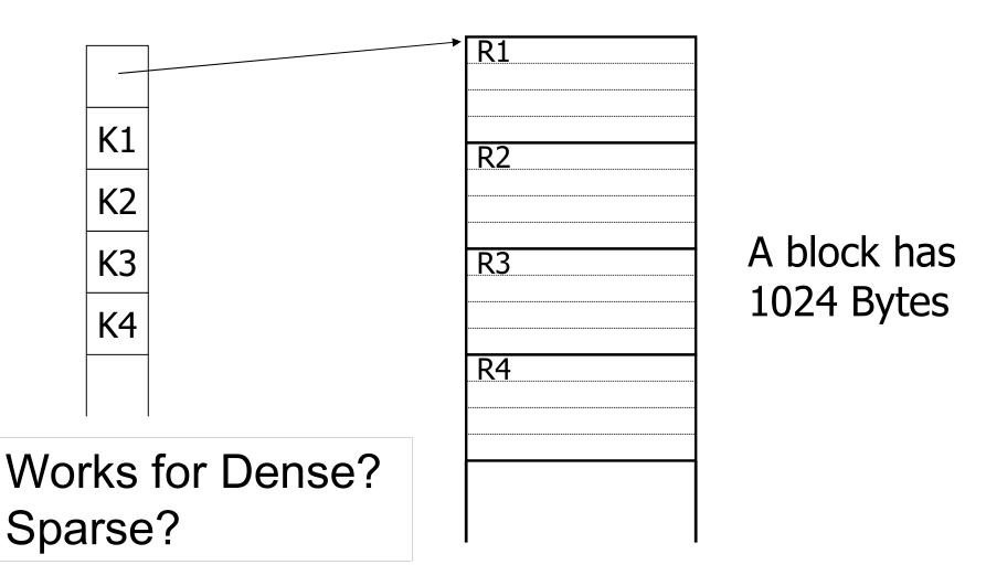
Find the K3 block by computing its offset: (3-1)1024 = 2048 bytes <sup>10</sup>
